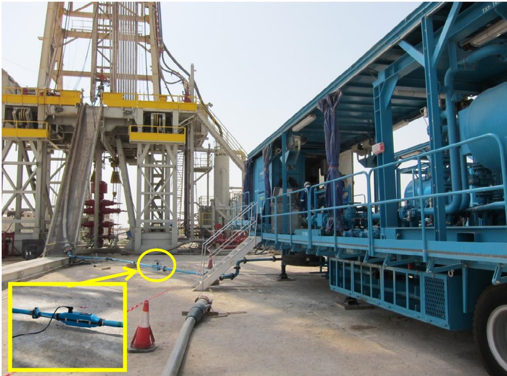
**Figure 14 SONAR Clamped-on to the Inlet flow line to a Portable Well Test Separator Package in Middle East**
