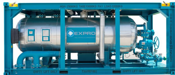
Shell and tube steam heat exchanger
