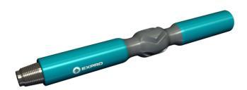
The **Cutting Bed Impeller (CBI™)** is a downhole drill string tool intended for use in deviated wells where excessive build-up of cuttings causes drilling problems, typically in hole angles greater than 30°. An integral drill string component, it consists of a short one-piece mandrel with no moving parts, and mechanical properties exceeding the specification of the drillpipe. Its hydraulic and mechanical dual acting mechanism removes cuttings beds inside the casing or in open hole.
