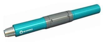
Intended for use in deviated wells where excessive rotary torque causes drilling and casing wear problems, the **Drill String Torque Reducer (DSTR™)** tool can reduce casing wear across the build section. For a given deviation profile, the applications program assists in maximizing the tool's performance by determining the deployment in the critical sections of the borehole.
