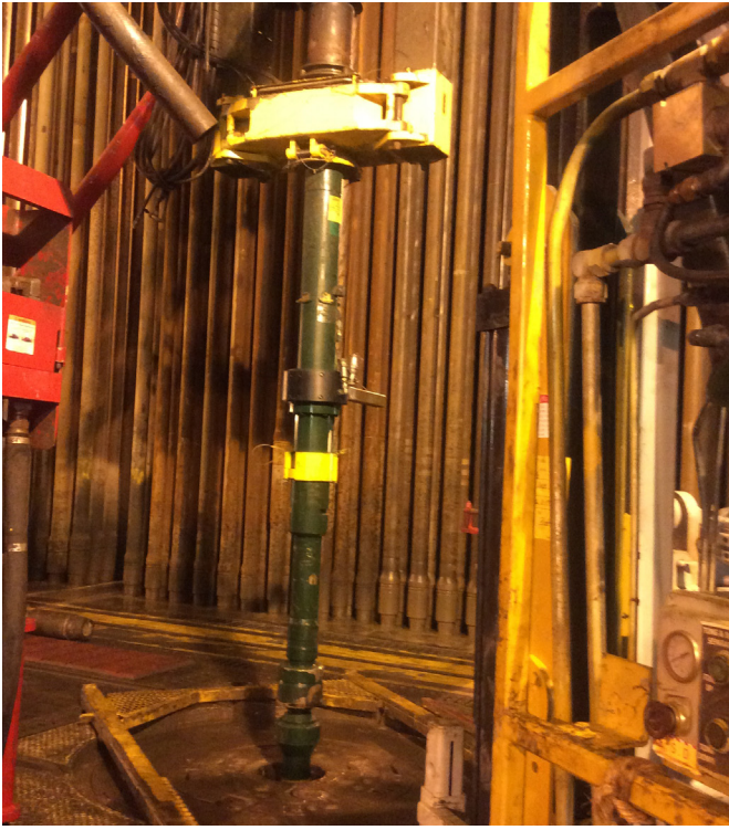
Figure 1. VERSAFLO tool in casing configuration.
