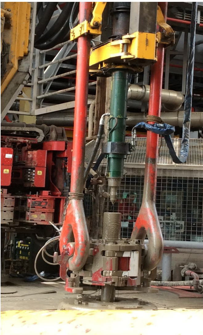
Figure 2. VERSAFLO tool in drill pipe configuration.
