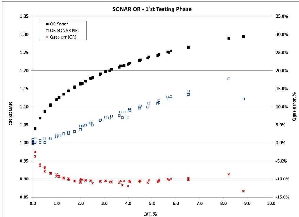
Fig. 4 - 1SONAR over reading versus LVF (1<sup>st</sup> Testing Phase)
