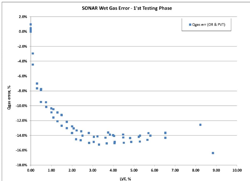
Fig. 3 - Wet Gas Error (SONAR vs. NEL) 1'st Testing Phase
