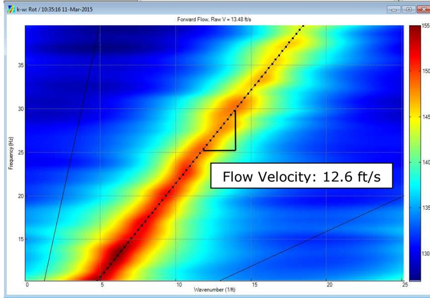
Fig.1 - SONAR Diagnostics: k- $\omega$  ridge
