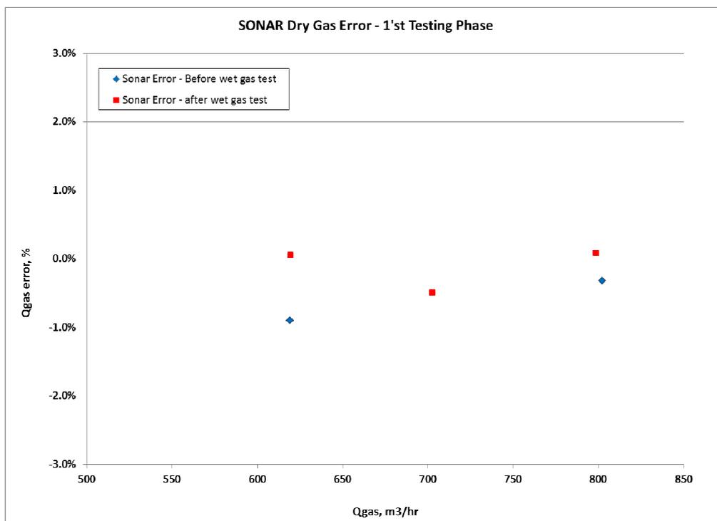
Fig. 2 - Dry Gas Error (SONAR vs. NEL) 1'st Testing Phase
