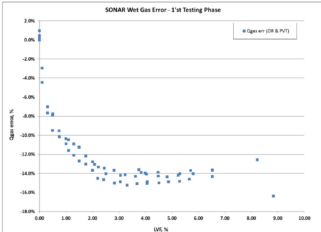
Fig. 3 - Wet Gas Error (SONAR vs. NEL) 1'st Testing Phase
