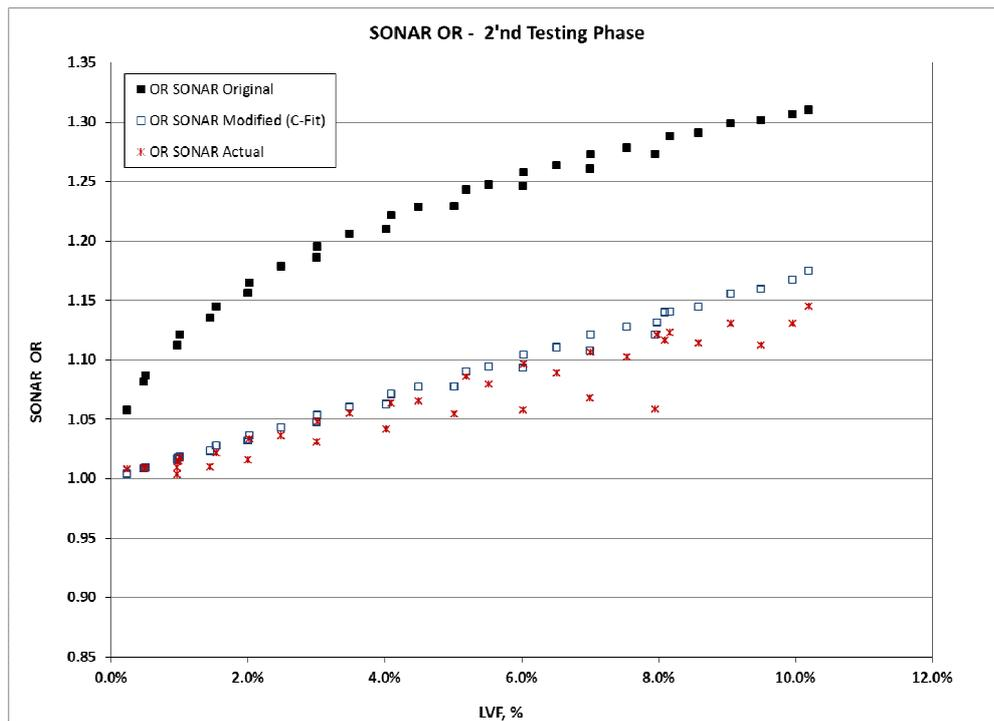
Fig. 7 - SONAR over reading versus LVF (2<sup>nd</sup> Testing Phase)
