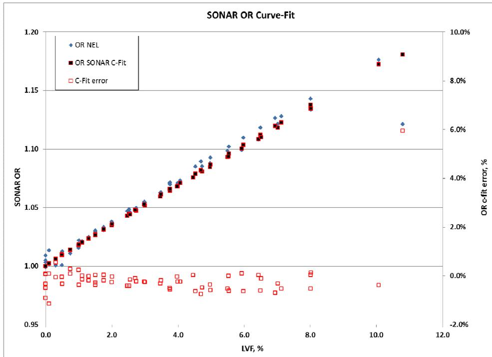
Fig. 2 - Over-reading curve-fitting for 12-in meter in wet gas flow
