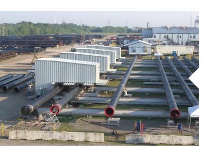
TENDONS are fabricated in several stages throughout the facility and our hex joint rack allows up to four (4) pipe-to-pipe welds simultaneously.
