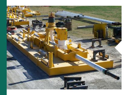
structural fabrication including pipe line end termination (PLET), transportation frames, shipping containers, and grillage can be performed in either of our open bays/tents, and/or at the bulkhead for ease of loadout onto barges.
