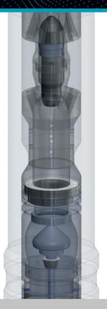
The Self-Filling poppet or flapper style-floats enable operators to accelerate trip times, saving up to 18 minutes per 1,000 ft run in hole by allowing self-filling and eliminating time-consuming top filling.
