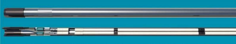
Expro Petrotech Tubing Conveyed Sampling Carrier is a unique tool for bottom hole sampling of HPHT wells. The 20K TCS Carrier can provide 4 x 540 cc (2.16 litres) of single phase reservoir samples. It may also be equipped with quartz memory gauges to measure downhole pressure and temperature.
