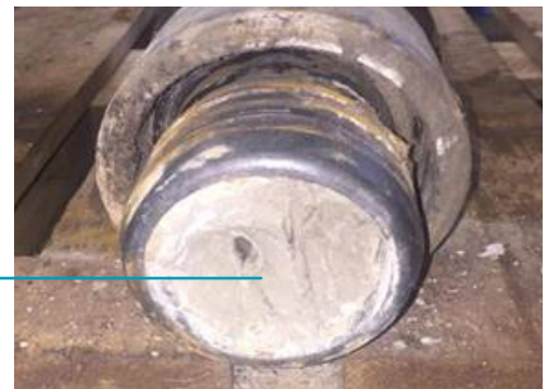
Cement sample recovered from beneath the latch in adapter ball seat of the SeaCure® system. A qualitative but definitive example of cement quality at the shoe.
