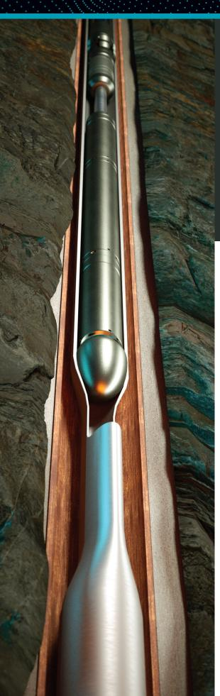
The Reform tool uses hydraulic pressure applied at surface to reform collapsed, oval, or restricted tubulars. As a targeted solution, it can remediate damage in vertical or horizontal wellbores where there is limited set down weight available for conventional swaging operations.
