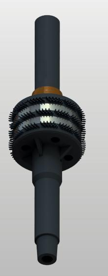
The Coretrax Riser Brush is an integral part of the drill string and is designed to clean the riser as the pipe is run into and pulled out of the well. It is stabilized slightly below the drift diameter of the riser to centralise the drill string.
