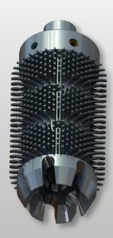
Setting a bridge plug successfully requires a clean setting area. The CX-DB (Drillable Brush) is made up directly to the plug or packer to clean and effectively prepare tool setting areas. Fluid is directed through the body of the Drillable Brush to support cleaning.
