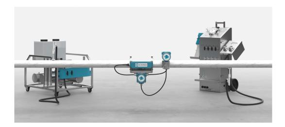
QPulse™ is a non-intrusive portable multiphase flow surveillance solution utilizing proprietary non-intrusive Sonar technology combined with a tracer technology. This innovative solution can be deployed for production testing and monitoring across the field and allows independent flow measurement of the three phases (gas, oil, and water). QPulse™ can be retrofitted on the existing production pipeline from the wellhead and therefore prevents the need to bypass the flow or interrupt production.
