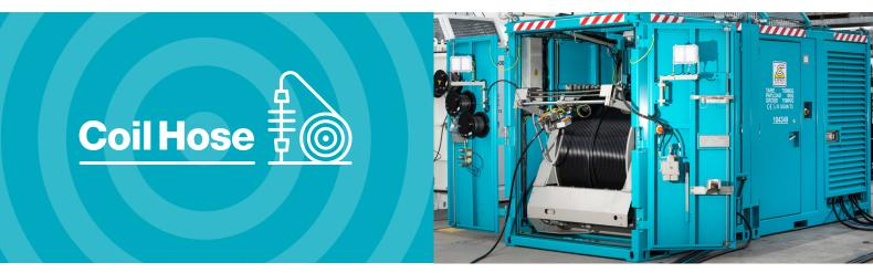
The CoilHose Light Well Circulation System is a hybrid well intervention system that combines the operational efficiency of a wireline deployment with the capability to perform a range of nitrogen and fluid pumping applications.
