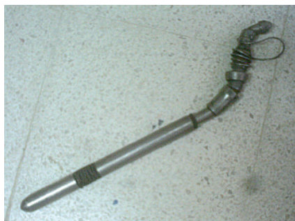
Deformed dummy valve which Expro recovered
