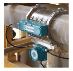
ActiveSONAR<sup>™</sup> is the next generation of clamp on sonar technology that used pulsed-array sensors, which measure flow rates in multiphase conditions
