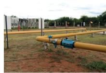
Expro carried out a pilot campaign to showcase the capabilities of the sonar flow measurement technology in wet gas multiphase application and demonstrated how this cost effective solution can be used in areas/applications where traditional production testing is not suitable or difficult to achieve.
