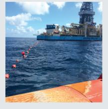
Environmental restrictions prohibit the amount of well tests that can be performed in the Gulf of Mexico. With a zero flaring restriction, hydrocarbons are transferred to tender-assist tankers during the test. The client had not performed such an operation in excess of 15 years and contracted Expro to manage both the well test design and well test operations.
