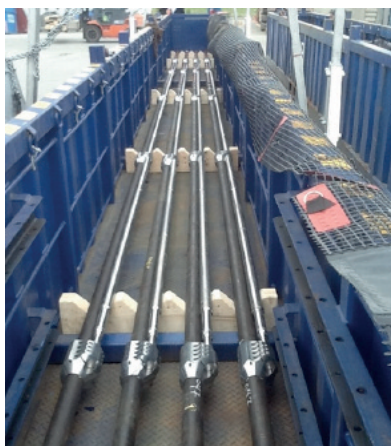
CaTS gauges mounted on the tailpipe
