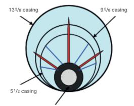
23/8 big hole gun with orientated bowspring de-centraliser
