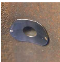
Orifice insert inside of tubing view
