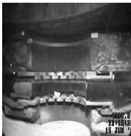
Snapshot from sideview camera looking at one of the VBRs (Variable Bore Ram)
