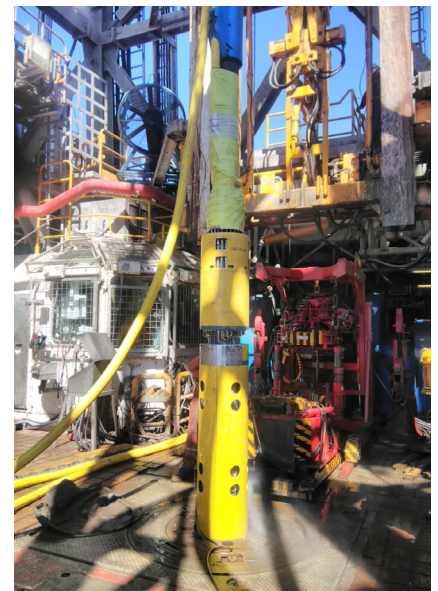
Fast Response Module being run in hole through the rotary table
