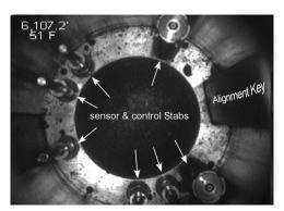
A deep-water operator in the Gulf of Mexico sought to ensure there was no debris on the shoulder of the sensor and control stabs in the tubing hanger of this subsea wellhead. Any debris could damage the stabs during the latch up which would require pulling the entire completion for repair. The image shows the shoulder free of debris and was used to align the connection before latching.
