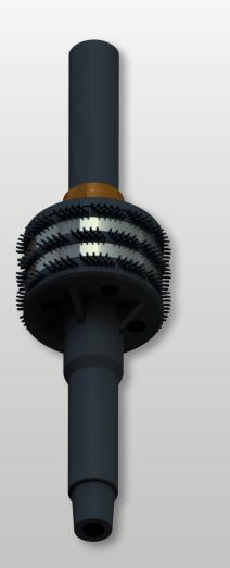
The Coretrax Riser Brush is an integral part of the drill string and is designed to clean the riser as the pipe is run into and pulled out of the well. It is stabilized slightly below the drift diameter of the riser to centralise the drill string.
