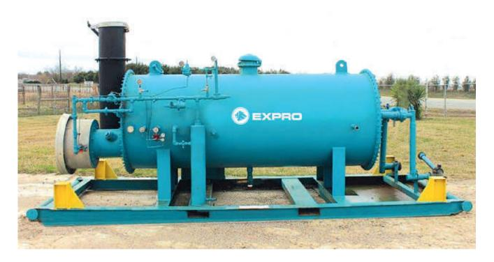
Expro can provide portable inline vaporizers form 250,000 to 1,500,000 BTU/hr with 2" inlet/outlet. These systems can be used to safely vaporize liquid products. Most commonly used in commissioning projects to either vaporize heavy products to gas to prevent nitrogen bubbles remaining in the product stream or to increase temperature of light products so it remains above the safe pipe metal temperature as it is introduced into the pipeline.
